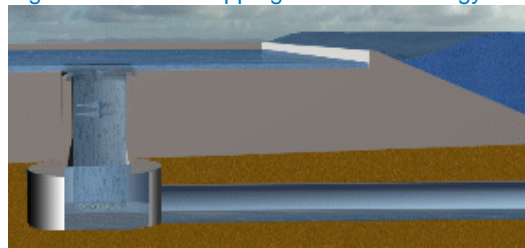
Figure 3-20: Overtopping fixed wave energy device
