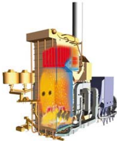
Figure 3-11: Bubbling Fluidised Bed (BFB)
