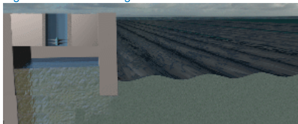
Figure 3-19: Oscillating water column fixed wave device
