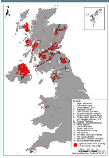
The UK contains over 500 km³ of silicate rock within extractable distance from the surface. The total carbon capture potential of this material is 430 billion tonnes. The constraints of the resource mean that not all of this potential would be exploitable. However, it should be noted that most of this potential exists in Scotland and N. Ireland (see Figure left). Yet, >22 and >2 billion and tonnes of CO<sub>2</sub> capture potential are present in England and Wales respectively. (Renforth 2012)
