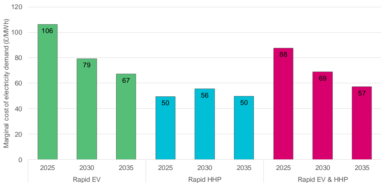
Figure 5 Rapid uptake of electric vehicles and hybrid heat pumps could decrease the cost of electricity
